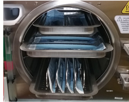
M11 Pouches w/ Pouch Rack & Trays Photo 8
