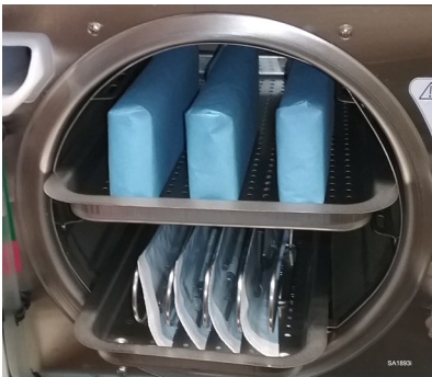
M11 Mixed load w/Cassette & Pouches Photo 11
