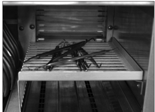
Figure 7D: Close up of improperly loaded half tray. Instruments should be placed so that they do not touch one another or extend over the tray periphery.
