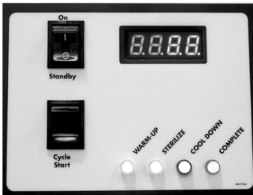
Figure 5: Control Panel for DDS 7000.
