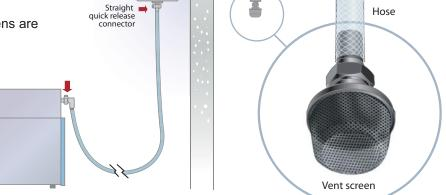
Please note: AAMI guidelines state that all EtO sterilizers should be vented (exhausted) through a dedicated vent line to the outside atmosphere directly or through an emission control system. The vent should not terminate within 25 feet (7.6m) of any building air intake source or near pedestrian or animal traffic, nor should it allow EtO release into or to reenter the building.
