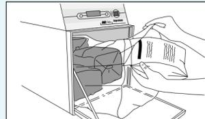
7. Place the gas-release bag in the liner bag on top of the items to be sterilized.
