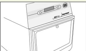
1. The machine will continue to purge the liner bag every 2 minutes until the operator unloads the sterilizer, closes the door, and presses the EXIT button. This allows for aeration within the cabinet. A timer will keep track of additional aeration.
