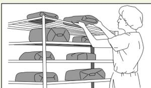
3. Plastic and rubber items should be aerated for an additional 24 hours at 68°F or warmer before use. Metal and glass do not require additional aeration. The room utilized for aeration must have at least ten air changes per hour.
