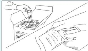
6. Remove one ampoule from the dispenser box. Unroll the plastic bag ("gas-release bag") in which it is sealed. Gently push the ampoule to the center of the gas-release bag.
