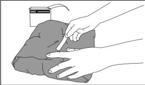
9. Apply one self-adhering chemical indicator to the outside of each package to be sterilized. Andersen Package Closure Indicator Strip (AN85/AN86) is a chemical indicator which verifies exposure to Anprolene gas. Unlike biological indicators they do not signify sterility.
