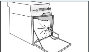
9. With the cabinet door open, press the PURGE button. The sterilizer will purge air out of the liner bag for 1 minute, 30 seconds.
