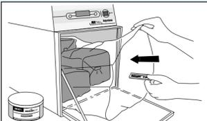
5. Place the appropriate biological (Steritest® AN80, AN2200, AN2203) or chemical indicator (Dosimeter) in the middle of the liner bag. If you cannot verify that the relative humidity is at least 35%, place a Humidichip inside a Humiditube (AN1072) and insert into the liner bag to ensure that the minimum humidity level is met.
