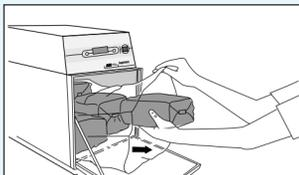
14. At the end of the purge cycle, the display will read "UNLOAD STERILIZER". The sterilizer will continue to purge the liner bag every 2 minutes until the operator unloads the sterilizer, closes the door, and presses the EXIT button.
