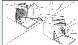
8. Insert the purge probe in the liner bag, placing the plastic ball towards the rear of the bag and the neck towards the opening. Then, gather the open end of the liner bag around the neck of the purge tube. Secure using the Velcro® strap.
