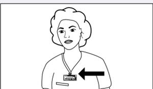
**SINGLE USE - PERSONNEL MONITORING** Airscan® Monitors (AN91, AN92, & AN93) measure personnel exposure to airborne concentrations of EtO. The badge is worn by the operator for the prescribed time (15 minutes to obtain the STEL level or 8 hours to obtain the TWA level). Badges are sensitive to smoke, perfume, and sunlight. These may provide a false reading. Refer to complete package instructions.
