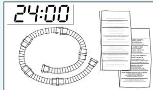
12. When sterilizing long lengths of plastic or rubber tubing greater than 3ft/1m, increase the cycle time to 24 hours. In these cases, a second ampoule may be necessary.
