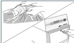
10. When the display indicates "BREAK AMPOLLE", carefully, so as not to puncture the sterilization liner bag, grasp the ampoule through the sterilization liner bag and activate it by snapping off the top. **CLOSE AND LOCK DOOR.**
