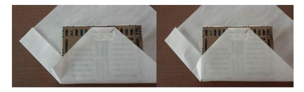
**Step 5** Fold over left corner and tape securely to first-fold wrap.
