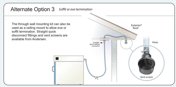
\* Please note: AAMI guidelines recommend all EO sterilizers be vented through a dedicated exhaut line to the outside atmosphere directly or through an emission control system. The vent should not terminate within 25 feet of any building air intake source or near pedestrian or animal traffic, nor should it allow EO release into or to reenter the building.
