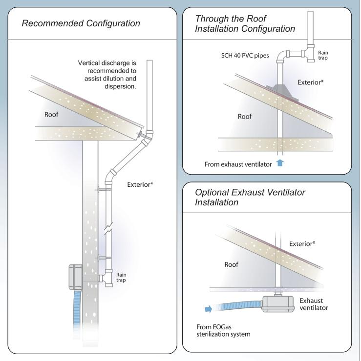
\* Please note: AAMI guidelines recommend that all EtO sterilizers should be vented (exhausted) through a dedicated vent line to the outside atmosphere directly or through an emission control system. The vent should not terminate within 25 feet (7.6m) of any building air intake source or near pedestrian or animal traffic, nor should it allow EtO release into or to reenter the building.
