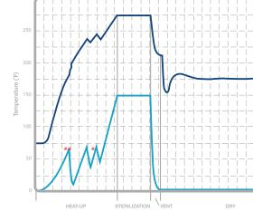
\*Three air removal purges. Electronic bellows purge air from chamber three times prior to sterilization for efficient air removal.
