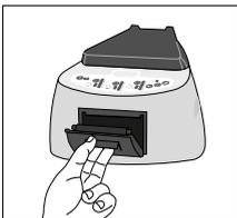
1. To replace the paper roll, pull the handle of the printer's door. Open the printer's cover and remove the spent roll.
