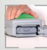
Sealed inside the unit during operation, the long-life lithium-ion battery is protected from moisture when decontaminating and will not disconnect or bump off while operating.
